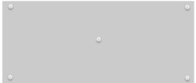
5 insulation fastener pattern (suspended ceiling/no external wind pressure applications)
